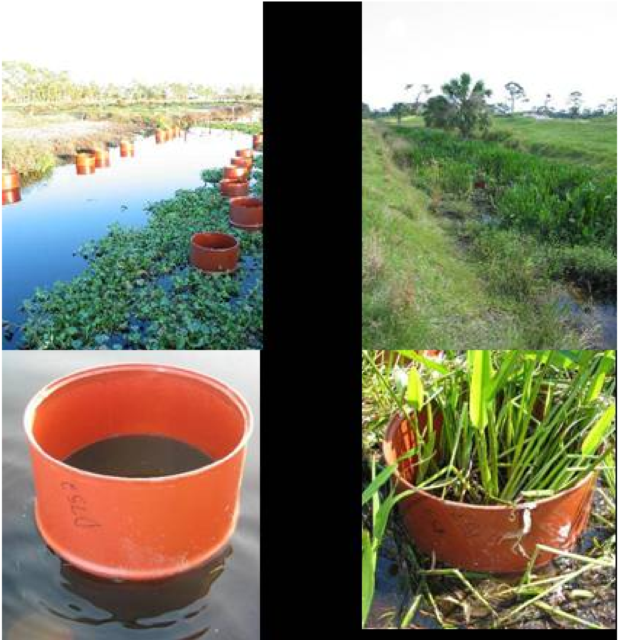
Figure 27. Mesocosm study for quantifying the effect of water retention on P retention in the two drainage ditches at flume sites 5 (left) and 4 (right) at the Pelaez Ranch (Collins, 2005).
